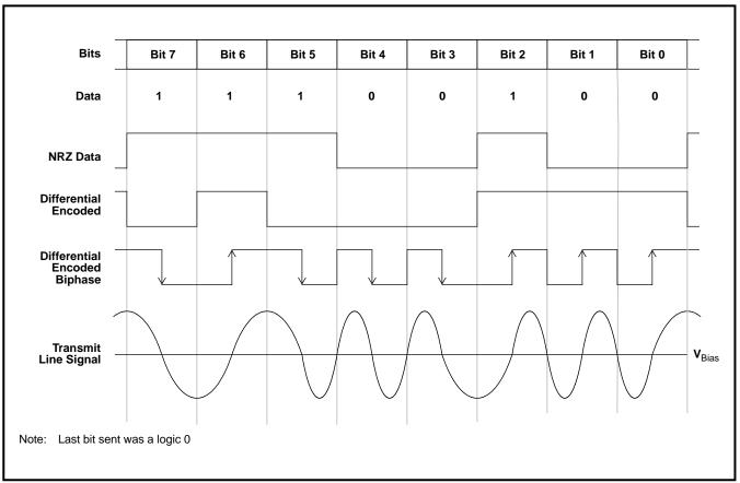
Figure 10 - Data & Line Encoding
