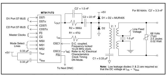
Figure 13 - Typical Connection Diagram - MAS/DN Mode, 160 kbit/s
