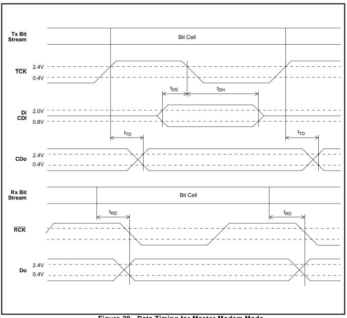
Figure 20 - Data Timing for Master Modem Mode
