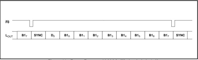
Figure 11 - Frame Format - 80 kbit/s (Modes 0, 2, 3, 4, 6)
