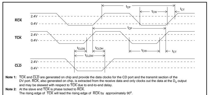
Figure 18 - RCK, TCK & CLD Timing For MOD Mode
