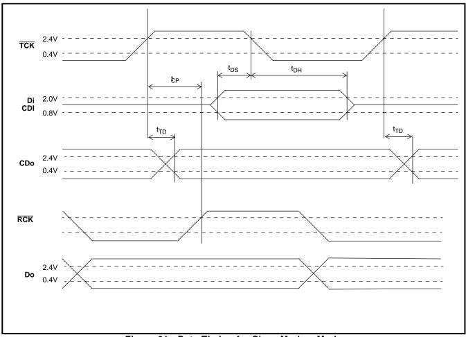
Figure 21 - Data Timing for Slave Modem Mode
