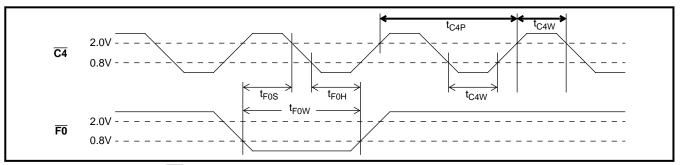
Figure 16 - C4 Clock & Frame Pulse Alignment for ST-BUS Streams in DN Mode
