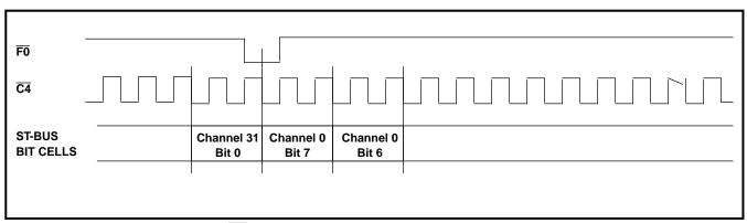
Figure 15 - C4 Clock & Frame Pulse Alignment for ST-BUS Streams
